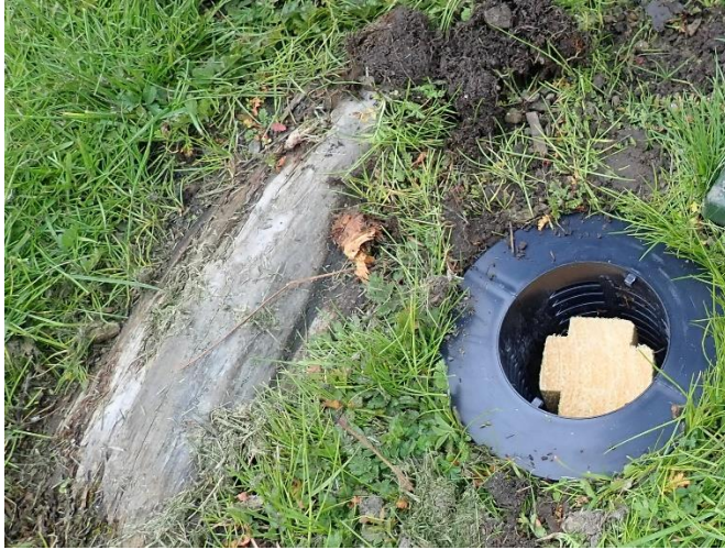
Figure 1. Exterra / Isophor EZE station containing wood monitoring blocks.
