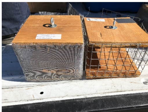
Fig. 4. An evaporation test cage with screen to exclude yellowjackets (left) and a bait cage to allow yellowjackets to enter and feed on the test bait (right).
