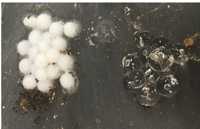
Fig. 3. Rehydration test with the final hydrogel bait. The hydrogel bait beads on the left are completely dried. When enough amount of water is provided, these dry hydrogel beads can be rehydrated (right), becoming palatable to foraging ants once again.
