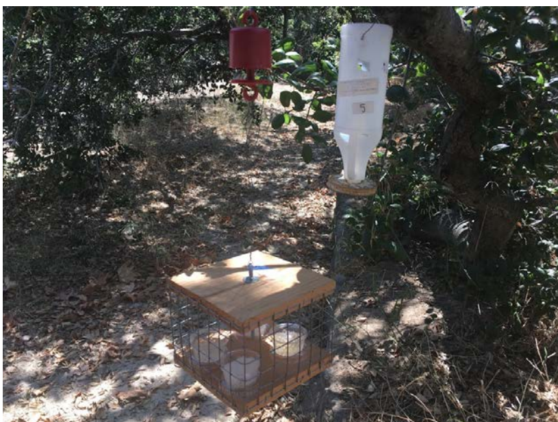
Fig. 16. Bait cups inside of a bait station. From lower left, clockwise, cups contained PAA, ALG, PAA, and ALG hydrogels. Note the ALG hydrogels are spherical, and PAA hydrogels have an irregular shape.
