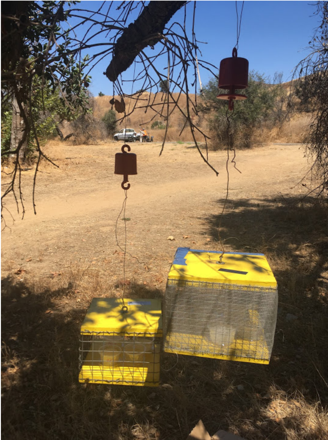
Fig. 17. A bait station (left) and an evaporation control station (right). Note the fine metal screen on the evaporation check station to prevent yellowjackets from foraging on the hydrogels.
