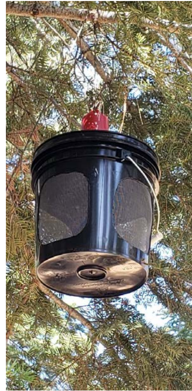
Fig. 7. The openings in the bait stations were covered with window screening to prevent yellowjackets from foraging on the baits or food attractants.
