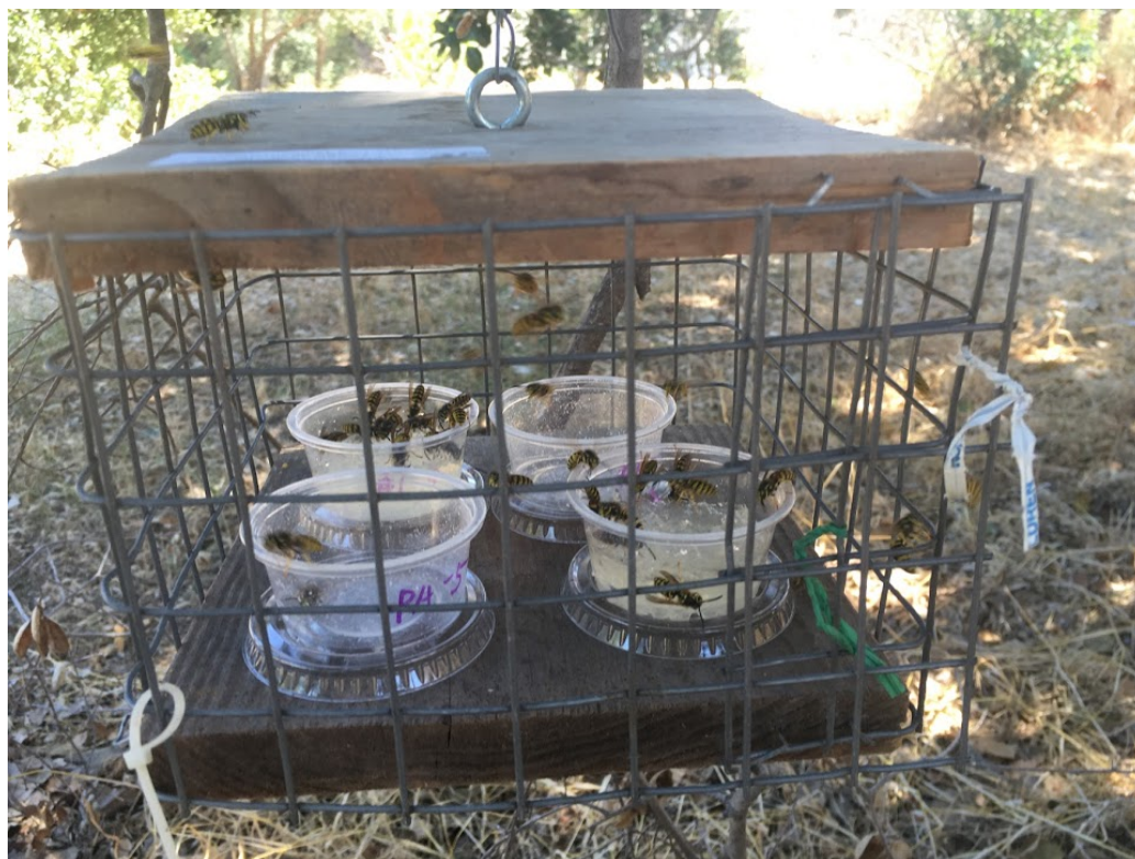
Fig. 26. Choice test at monitoring location #1. The photo was taken about 2 hours after the initial setup. From the lower left, clockwise, cups contained PAA, ALG, PAA, and ALG hydrogels. Note both PAA cups were nearly empty while ALG cups still had most of the ALG hydrogel beads.
