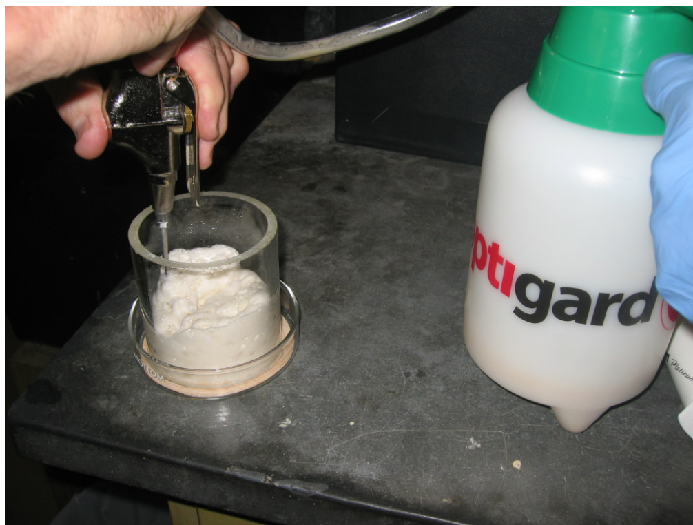
Fig. 3. Applying the foam by way of the Optigard ZT Foamer Kit into the glass cylinder resting on a balsawood disk. The cylinder is removed when the foam breaks, leaving a pool of liquid covering the disk.
