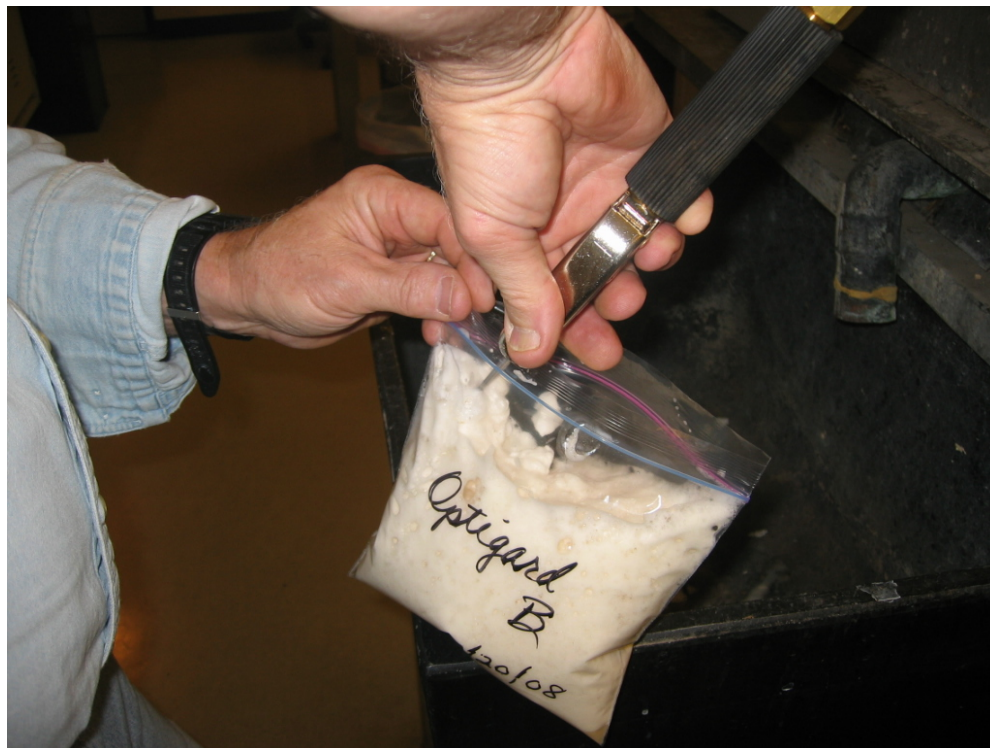
Fig. 2. Loading foam into a 730-ml plastic bag.
