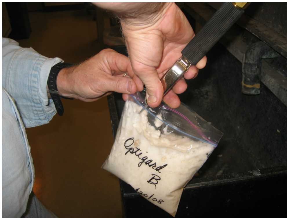
Fig. 2. Loading foam into a 730-ml plastic bag.
